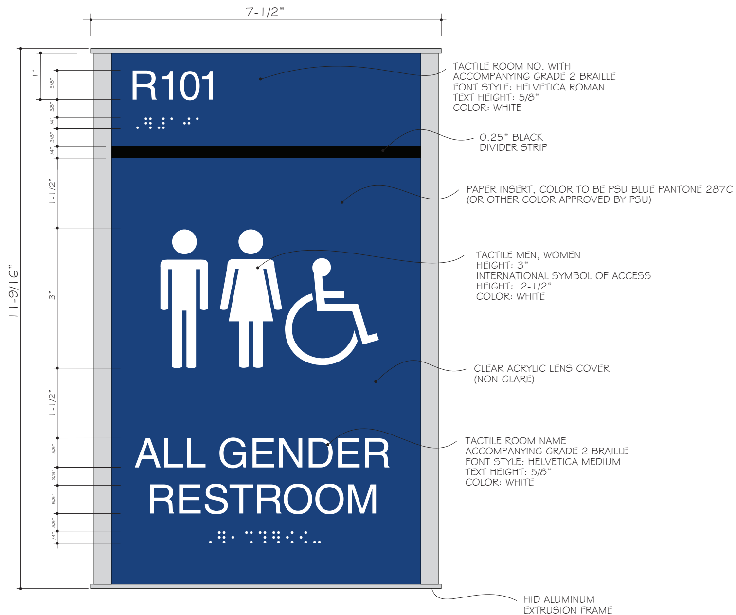
1 Elevation - Sign Type WMP-F711 Scale 1/2" = 1" Gender Neutral Restroom ID (Accessible)
